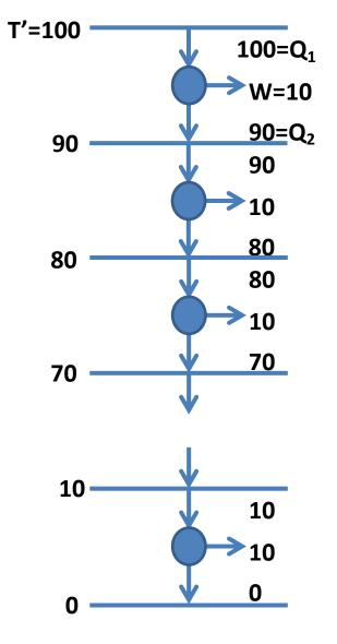
Kelvin derived a temperature scale not based on the expansion of gases or liquids, but based on Carnot's heat engines. Consider a series of Carnot engines, each producing the same amount of work, say 10 units, as in the figure.
