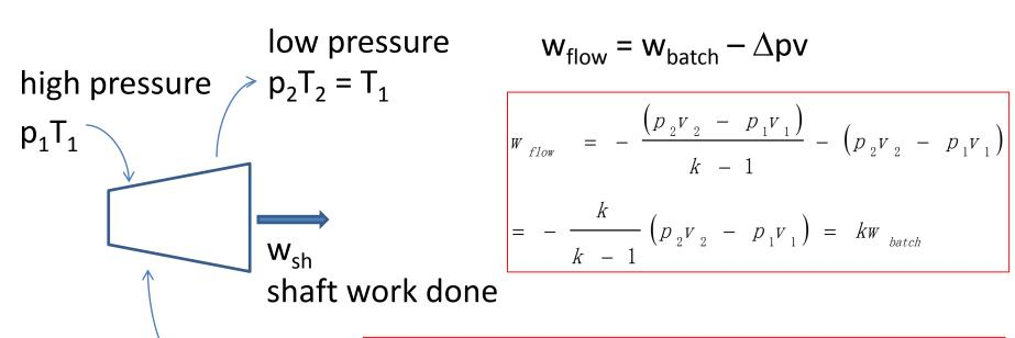
$$\vec{W} = \frac{kp_1\vec{V_1}}{k-1} \left[ 1 - \left( \frac{p_2}{p_1} \right)^{(k-1)/k} \right] = \vec{n} c_p T_1 \left[ 1 - \left( \frac{p_2}{p_1} \right)^{(k-1)/k} \right]$$
