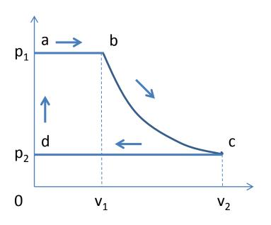
• a-b Introduce 1 kg of high pressure gas at  $p_1$  and of volume  $v_1$ .
