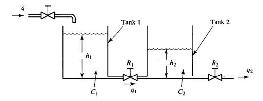
The capacitances of tank1 and tank2 are  $C_1$  and  $C_2$ , respectively. The resistance of the valve between the tanks is  $R_1$  and that of the out flow valve is  $R_2$ .
