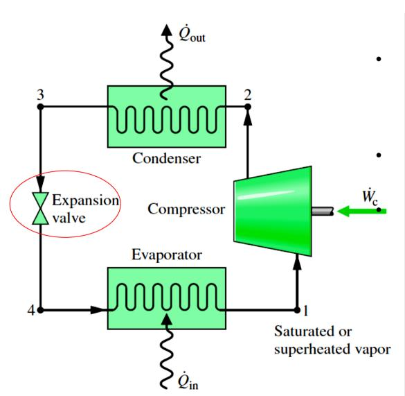
The expansion produces a relatively small amount of work compared to the work input in the compression process.
