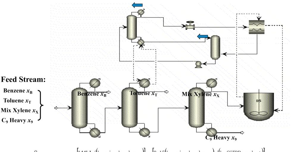
$$\frac{Q_{\text{Crystallization}}}{Q_{\text{Toluene}}} = \frac{\left[144 \text{kJ} / (\text{kg mixed xylenes})\right] \times \left[0.15 (\text{kg mixed xylenes}) / (\text{kg CSTDP product})\right]}{\left[319 \text{kJ/(kg toluene})\right] \times \left[0.70 (\text{kg toluene}) / (\text{kg CSTDP product})\right]} \approx 0.097$$
