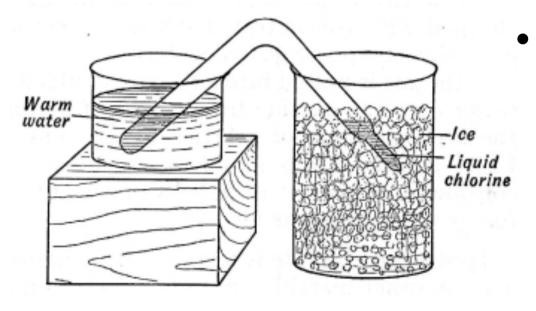
A faint yellow atmosphere filled the tube and, after some time, yellow liquid chlorine formed in the cool end of the tube.
