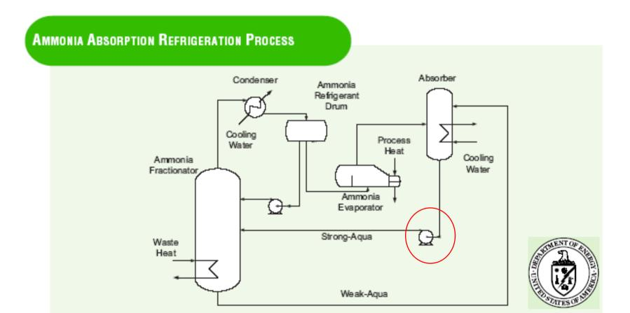
Ammonia absorption refrigeration conceptual flow diagram.
