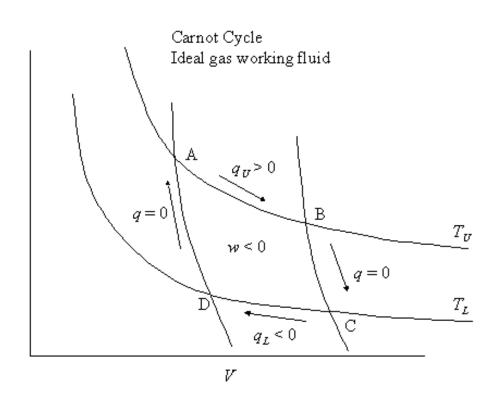
From point A, the system undergoes an isothermal expansion at temperature,  $T_{ij}$ , to point B. In this isothermal expansion the system absorbs heat from the upper heat bath  $(q_{IJ} > 0)$  and does work on the surroundings (w is defined as work done on the system so  $w_{AB}$  < 0).
