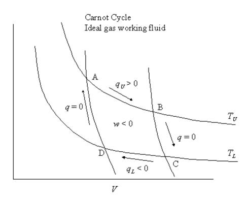
At point D the system is again isolated from the heat baths and compressed adiabatically to point A. In this adiabatic compression the heat, of course, is zero and the work is positive  $(w_{DA} > 0)$
