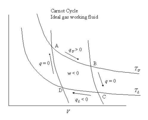
The curves labeled  $T_{ij}$ and T<sub>1</sub> are isotherms.  $T_{ij}$  is the temperature of the upper temperature heat bath (reservoir) and  $T_i$  is the temperature of the lower temperature heat bath. The two steep curves, BC and DA, are adiabatic curves.
