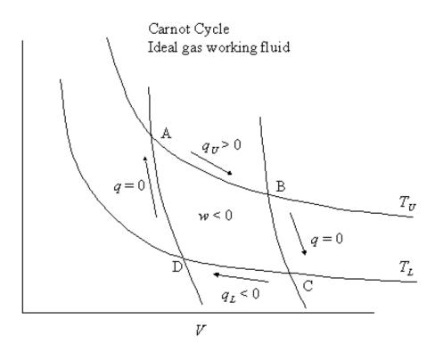
From point B, the system is then isolated from the heat bath and is expanded adiabatically to the point C. There is no heat in this adiabatic expansion, but the work for this step is also negative ( $w_{BC}$  < 0).
