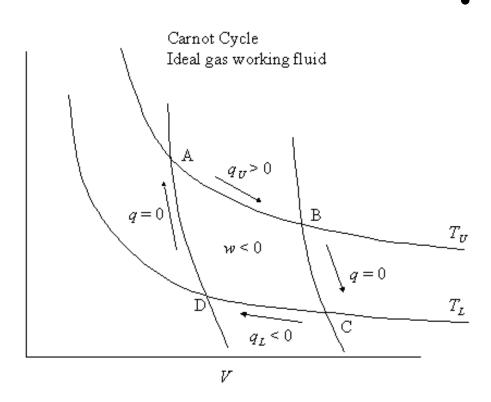
At point C the system is placed in contact with a heat bath at  $T_i$  and undergoes an isothermal compression to point D. For this segment of the cycle  $q_i < 0$  and  $w_{CD} > 0$ because the surroundings are now doing work on the system and heat is being dissipated to the heat bath at T,
