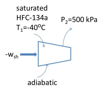
Find the work needed to compress adiabatically and reversibly to 500 kPa a stream of saturated HFC-
