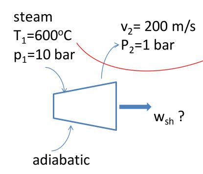
$$h_2 + \frac{v_2^2}{2} - h_1 = q^0 - w_{sh}$$
